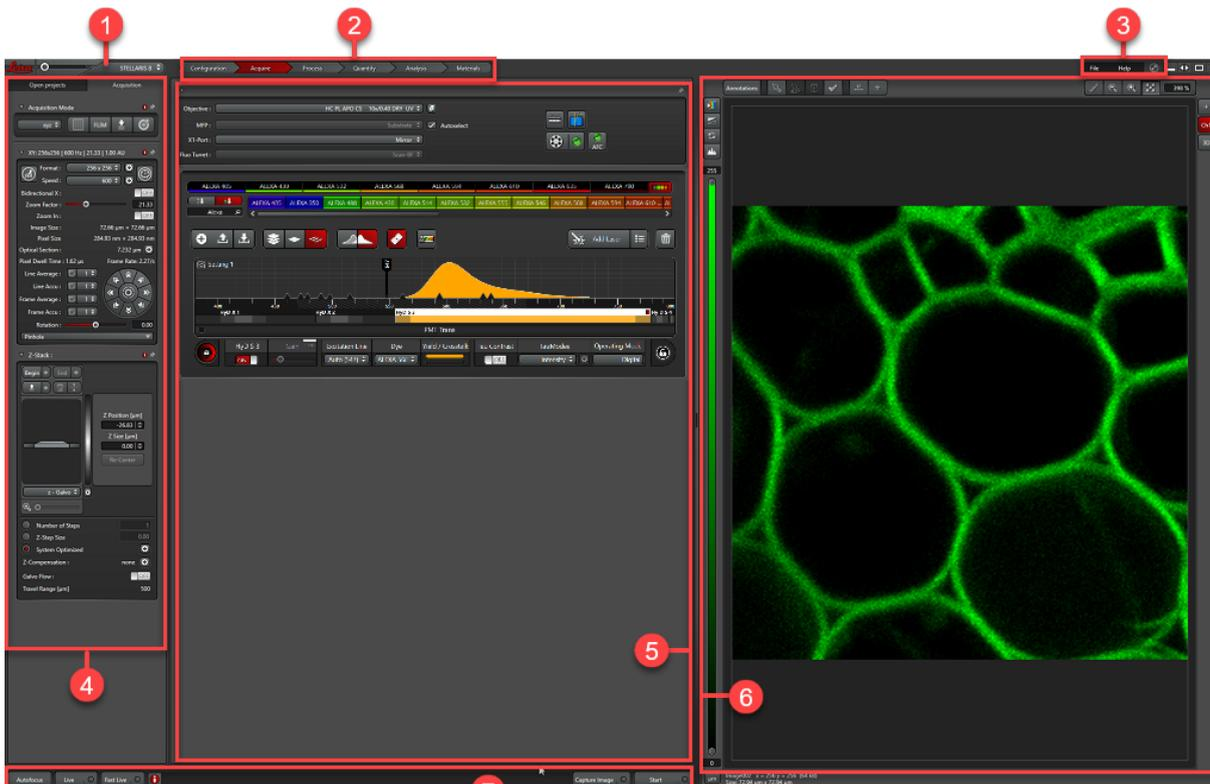
**1&4) Scanner parameters (XY) and Z stack controls. 2) Workflow steps 3) Help & support 5) Beam path parameters & Channel settings 6) Image viewer 7) Acquisition toolbar.**
